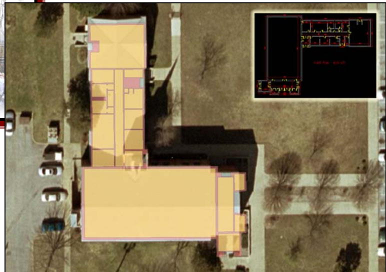
Example of SDSFIE compliant building footprint with floor plans in GIS. Data imported from CAD files for every structure on base.
